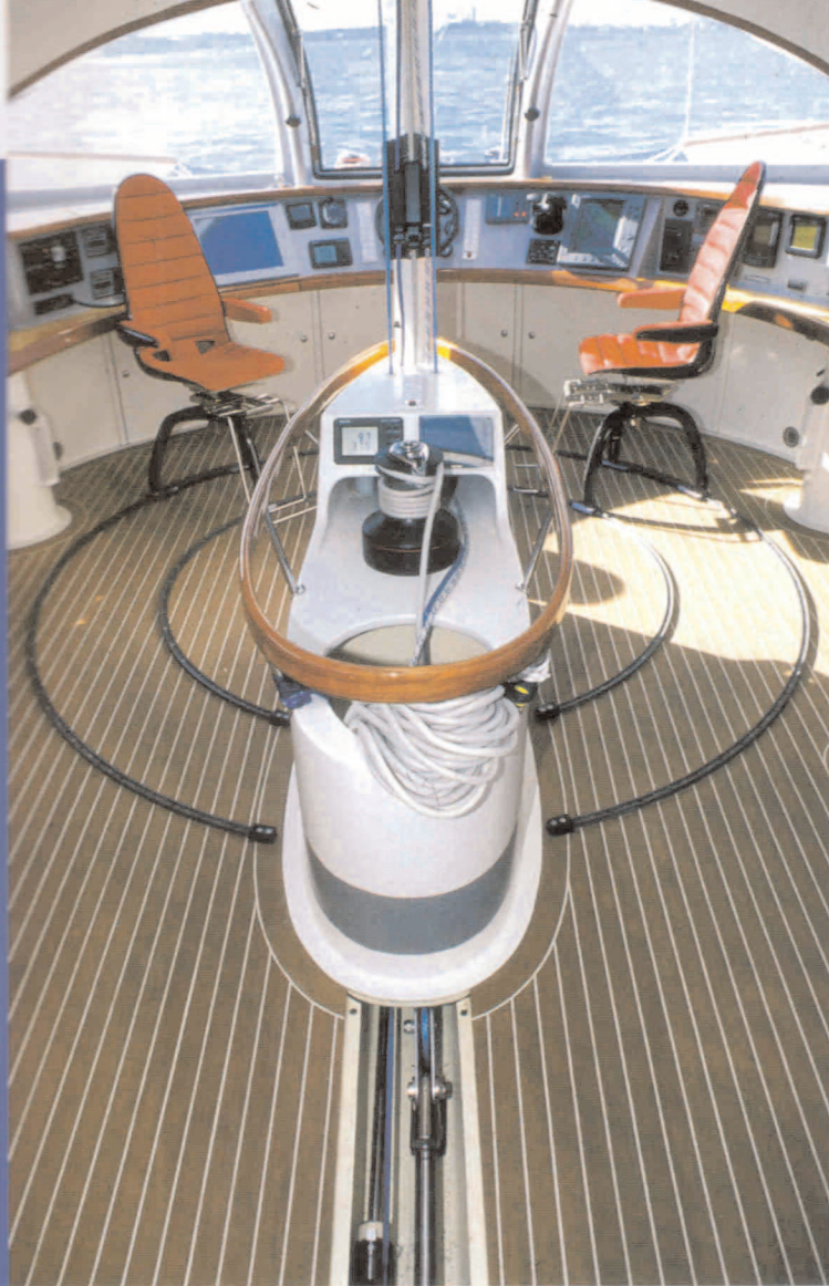
Above: mission control. The central pod houses the main halyard and reefing lines. Above right, top: the well equipped gas-free galley lies opposite the saloon seating. Bottom: primary sheet winches may be inside but the crew have a good view
